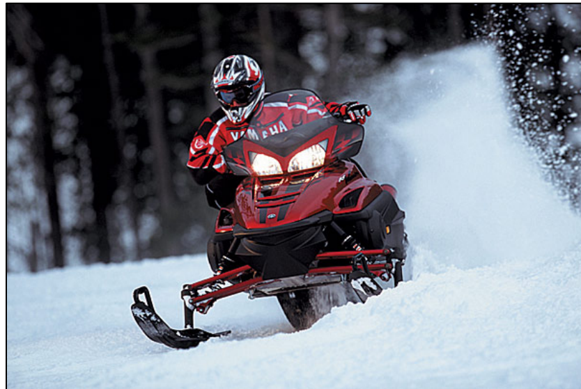
Photo 1.11 A snowmobile's skis, track, and suspension all contribute to mogul formation
